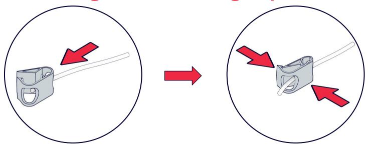
Thread the rope under the pulley and then pass through a Rope Clamp.
